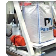
Vibrating table provides a compacted material by means of vibration ensuring a maximum of volume reduction of the material in the big bag
